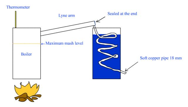
From the top of the lyne arm a soft copper tube is connected that is in a barrel of water. The barrel can be made of plastic and doesn't have to be as large as the boiler, 30 litre barrel is enough if cooling water is constantly fed to the barrel.
