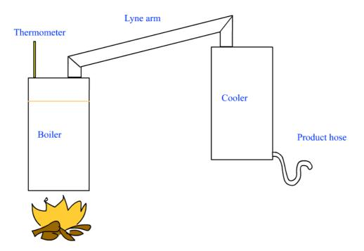
Instead of mounting the lyne arm onto the side of the barrels the lyne arm can use the barrel connectors on the lid. A common type of oil drum has a 2" tap onto the lid. Use a connector to fasten the lyne arm to the 2" tap.
