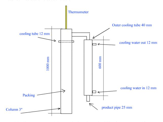
Material, either copper or stainless steel. The column should be about 3" to provide enough speed to a 200 litre boiler. One metre high is enough to give rather good separation.
