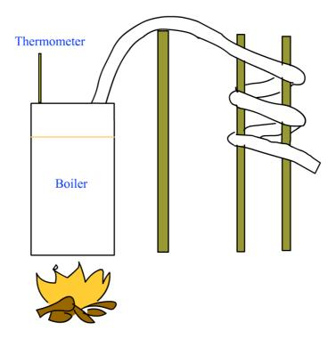
Flexible stainless steel or aluminium hoses are used in the car industry for instance. A 2" hose about 10 metres suit fine as an air cooled condenser. Using air alone as a cooling medium for a condenser limits the cooling capacity but makes the installation simple. Drawback is that the distillation takes longer time. Simply don't top up the boiler with mash to avoid the distillation run to take to too long time. The cooling becomes much more efficient if hose is exposed to breeze.
