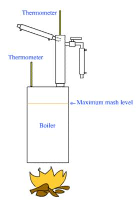
Boiler, can be made of an oil drum for instance ( 200 litres/50 US gallon or smaller) and be heated by fire, steam, with a gas burner or an electric heater.
