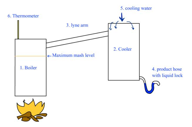
**Important!** This description is for fuel ethanol stills, if the stills are going to be used to provide drinkable alcohol as well all parts need to be food grade quality and ethanol resistant. Do not use solder containing lead, or galvanized pipes since it will be poisonous.
